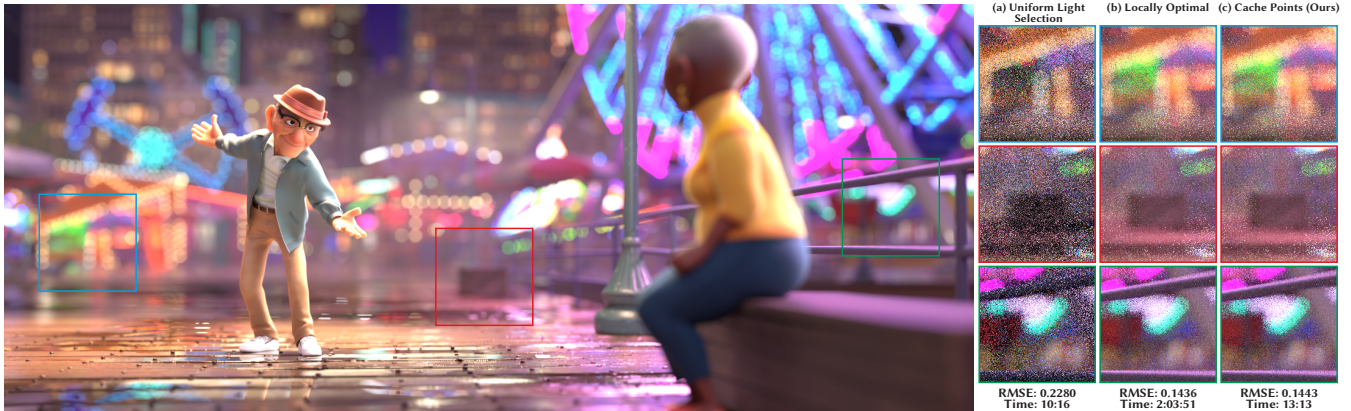
Figure 1: A production scene from Us Again containing 4881396 light sources (analytical lights, emissive triangles, and emissive volumes), rendered using 32 samples per pixel with uniform light selection (a), locally optimal light selection (b), and our cache points system (c). Uniform light selection produces a faster result but converges poorly, while building a locally optimal light distribution per path vertex produces a more converged result but is much slower. Our cache points system (c) produces a noise level similar to (b) while maintaining performance closer to (a). To clearly show noise differences, this figure does not include the post-renderer compositing that is present in the final production frame. © 2024 Disney
