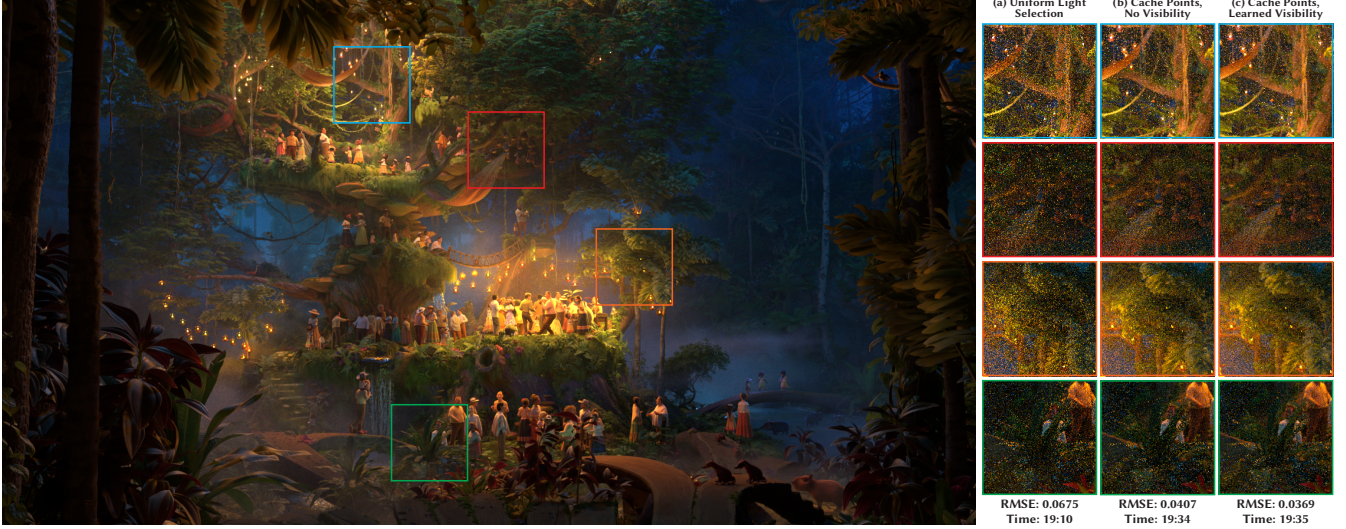
Figure 5: A production scene from Encanto containing 4406 light sources (analytical lights, emissive triangles, and emissive volumes) with complex occlusion, rendered using 32 samples per pixel with uniform light selection (a), cache points with no learned visibility estimates (b), and cache points with learned visibility estimates (c). In this scene, using learned visibility estimates results in a 9.3% improvement in RMSE for little to no additional render time. © 2024 Disney
