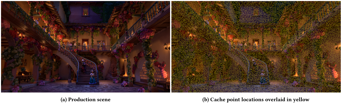
Figure 3: A production scene from Encanto (a) containing 38720 light sources (analytical lights, emissive triangles, and emissive volumes) sampled using cache points (b). Initial cache point placement suggested 388888 candidate cache point locations, which were pruned down to 48364 final cache point locations. For illustrative purposes, in this figure we only show cache point locations on surfaces; in actuality we also populate cache points volumetrically in space to support light sampling in participating media. © 2024 Disney
